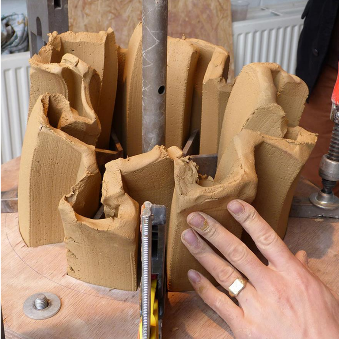
Figure 21. Ceramic Extrusion From Bottom to Top
