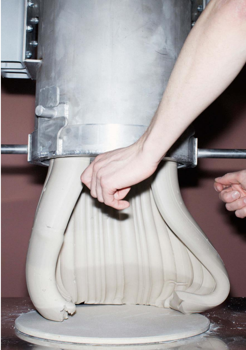
Figure 20. Vertical Extruder From Above Cutting Module
